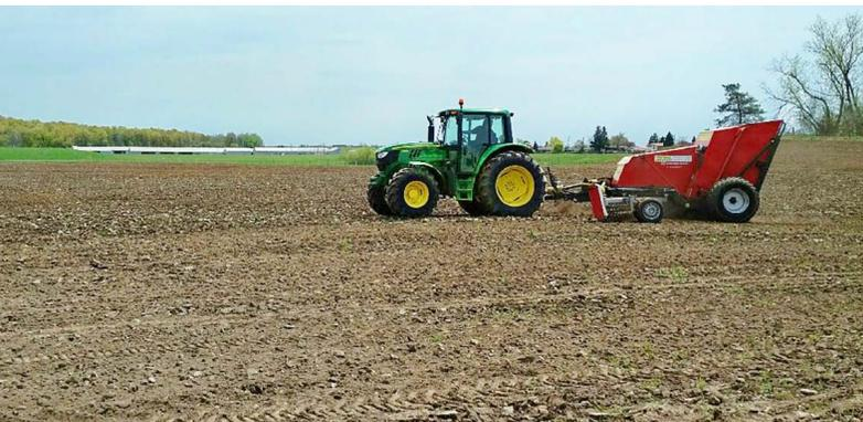
Once topsoil is reapplied to areas undergoing rehabilitation, special equipment is used to bring to the surface and remove excess stones.
